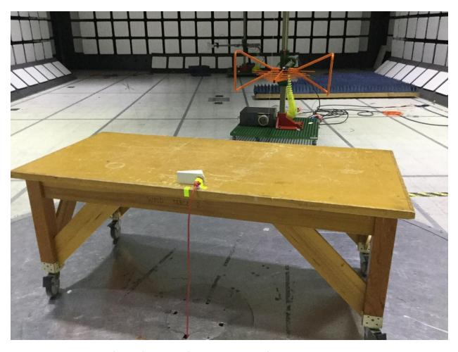
Foam was not placed in front of the table for measurements from 30 MHz - 1 GHz.
