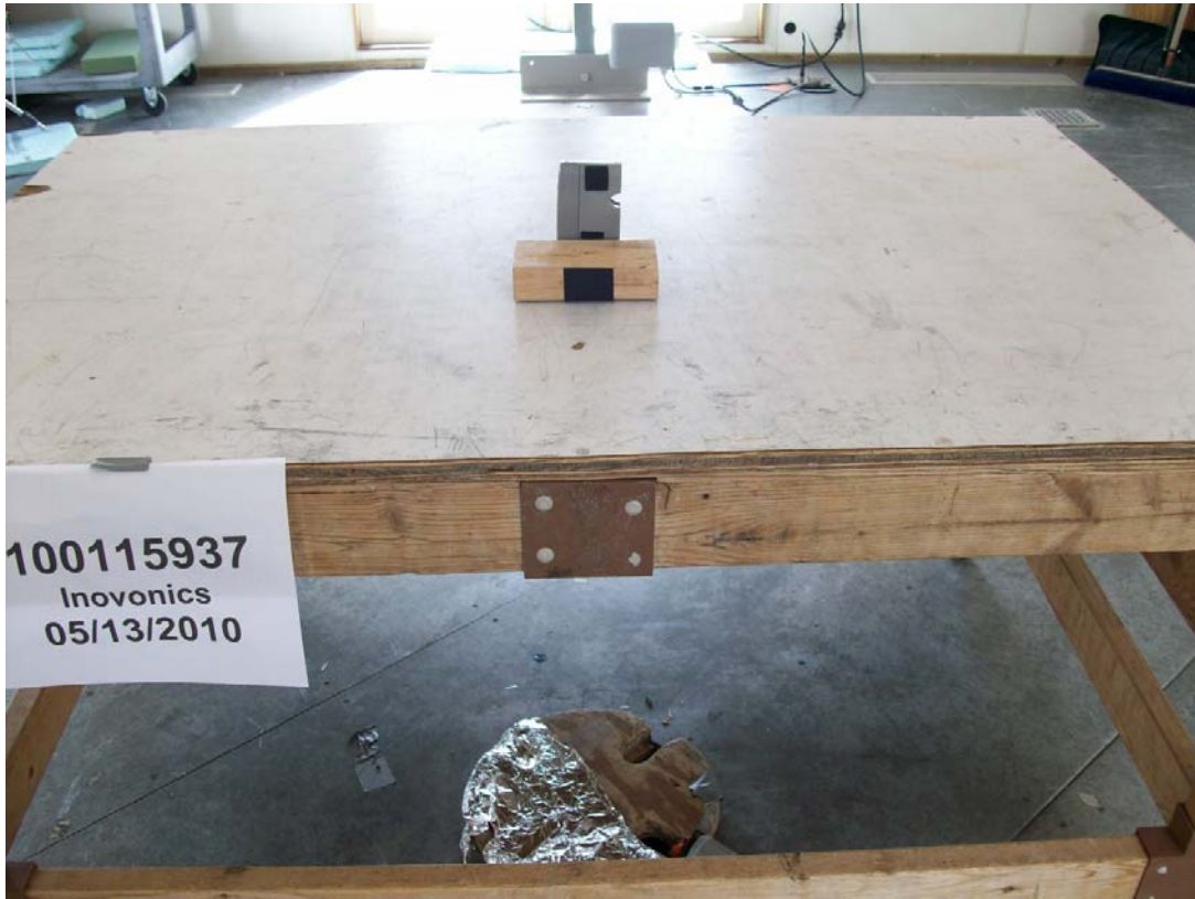
Radiated Emissions Test setup – Rear View
