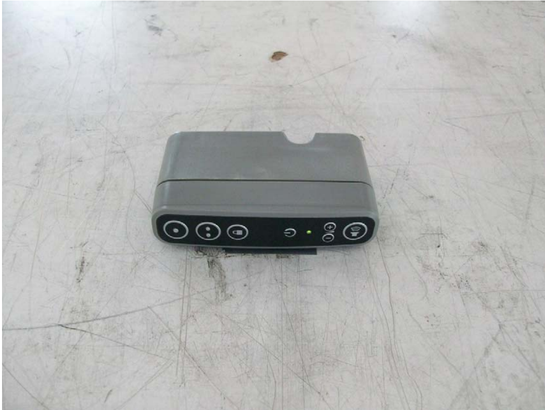
Test setup – Axis 1 (EUT Flat on Table)
