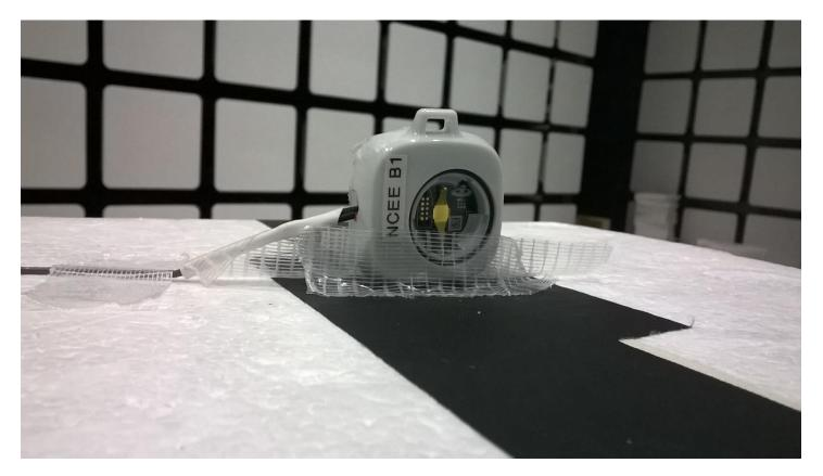
Figure 2 - Radiated Emissions Test Setup, 1 – 19 GHz
