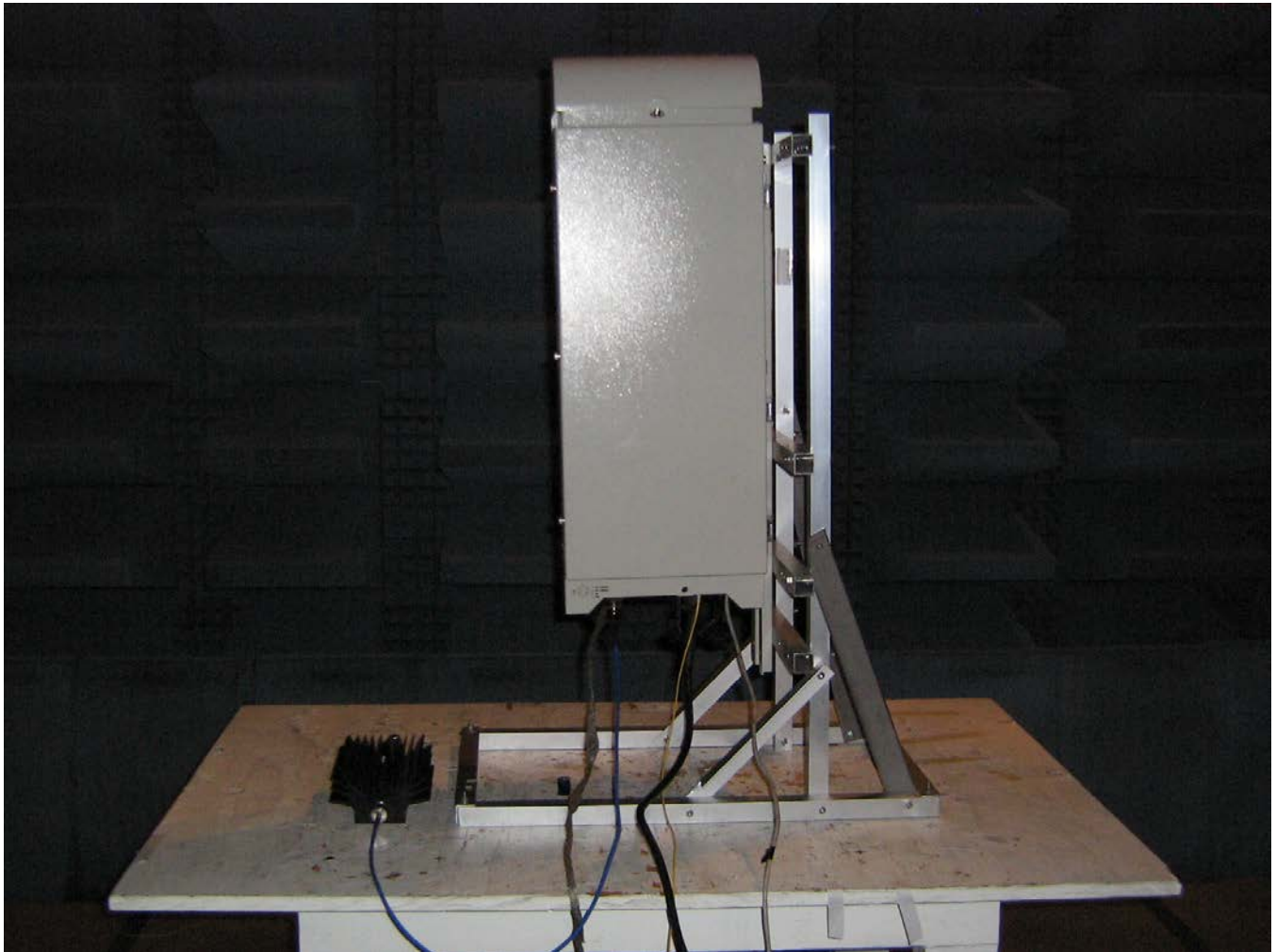
Picture 2: Radiated Emission test setup in Semi Anechoic Chamber
