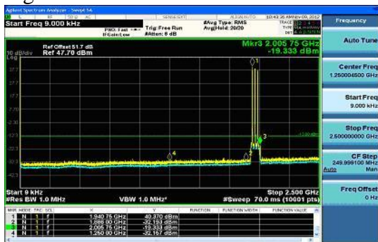
Fig. C1. CDMA 2000 emission 9kHz-2.5GHz
