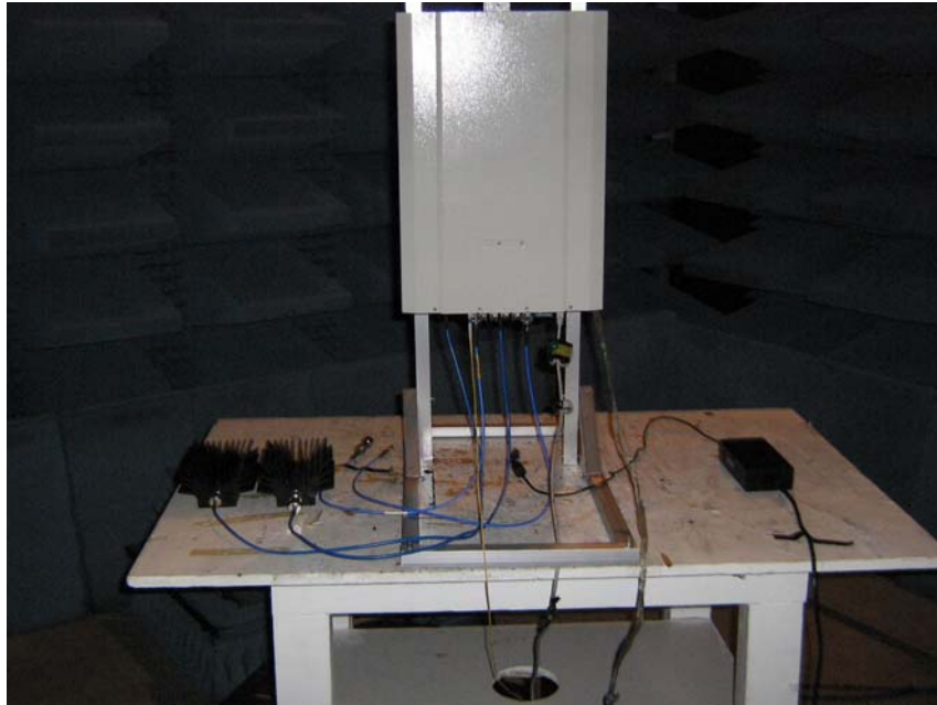
Picture 1: Radiated Emission test setup in Semi Anechoic Chamber
