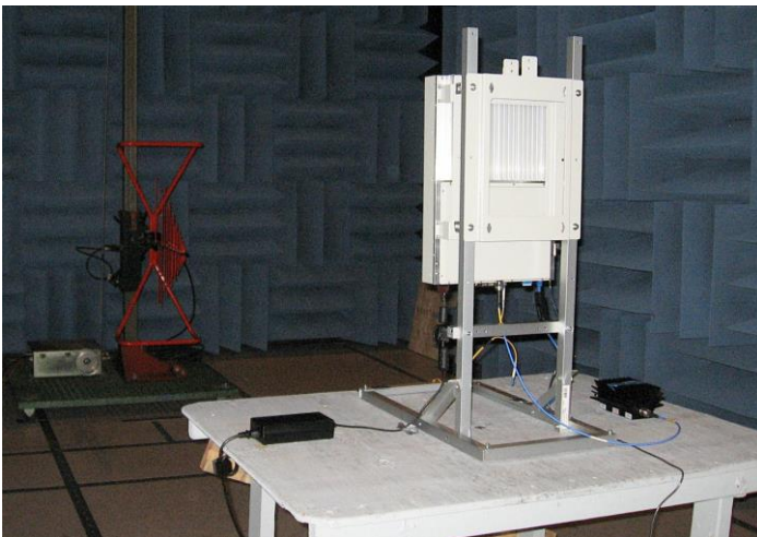
Picture 2: Radiated Emission test setup in Semi Anechoic Chamber
