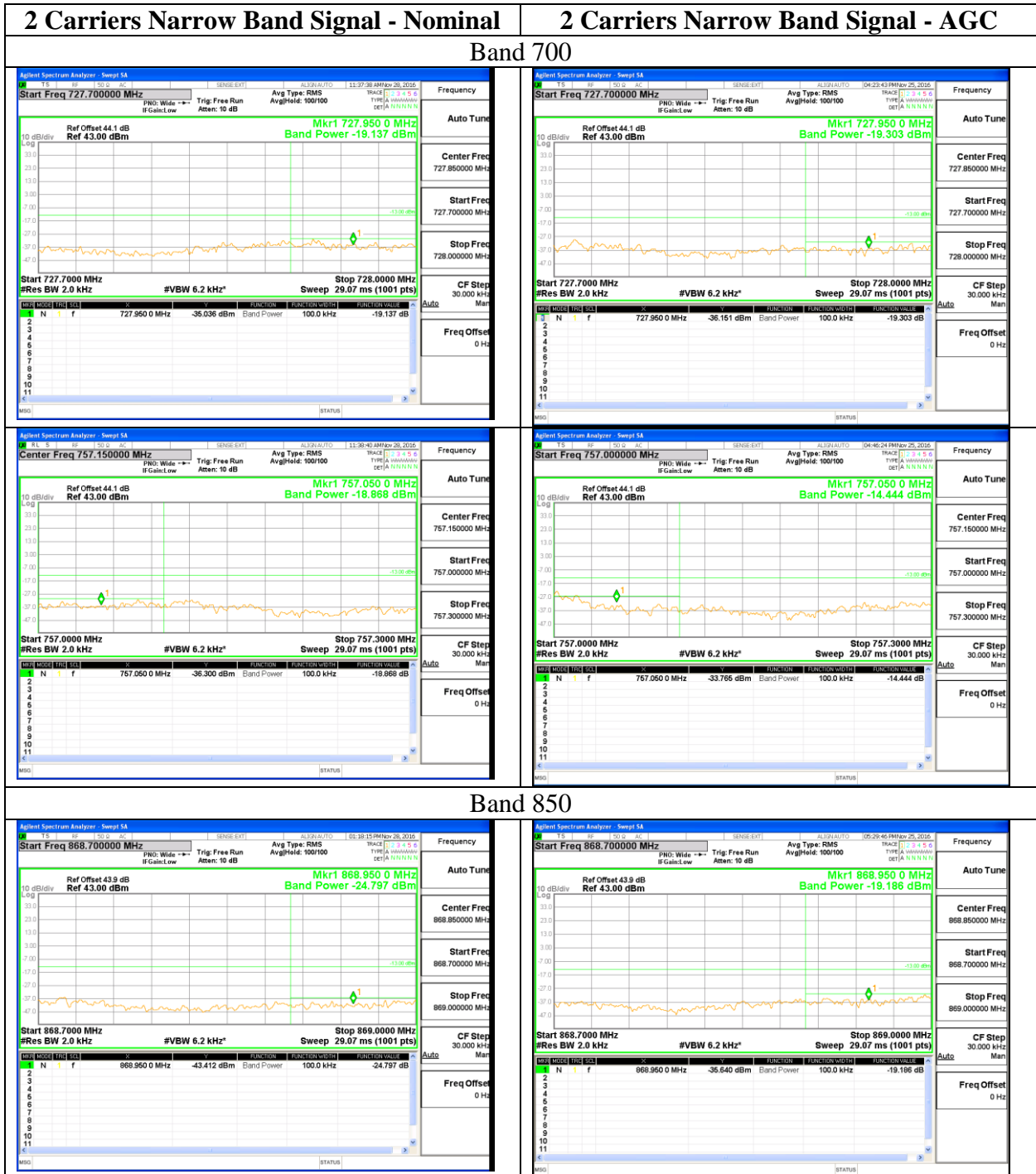
Figure 6-3 Out-of-band Emission in 300kHz or 3GHz Range – 2 Carriers Narrow Band Signal Applied on First or Last Channel in the Appropriate Operating Band
