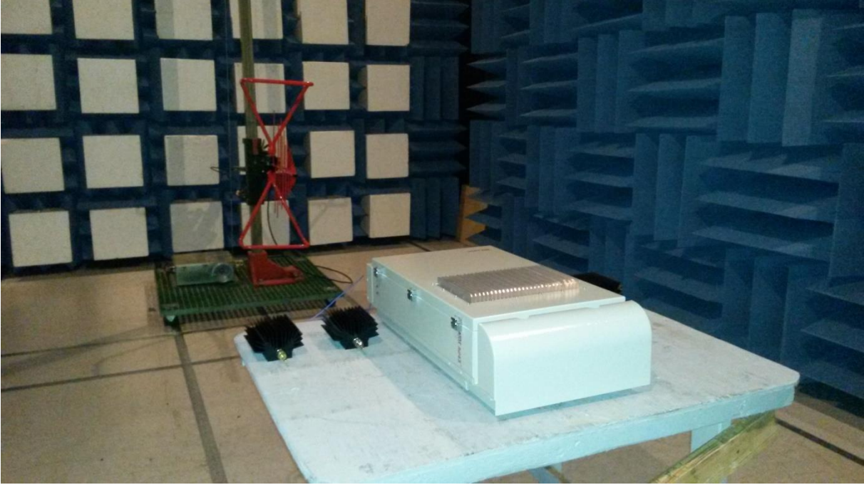
- Test Setup under 1GHz with JB1 Antenna.
