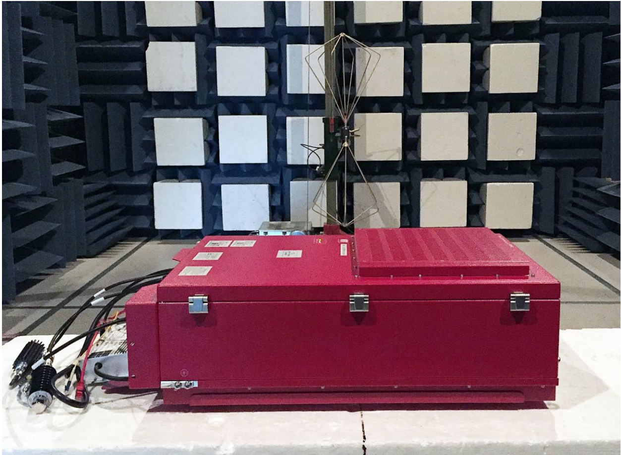
Figure 2: Radiated Emissions (30 to 300MHz) Test Setup: Emissions on Cabinet
