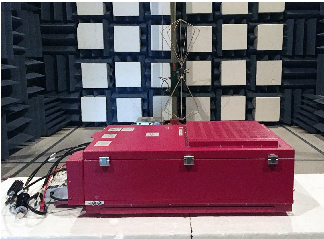
Figure 2: Radiated Emissions (30 to 250MHz) Test Setup
