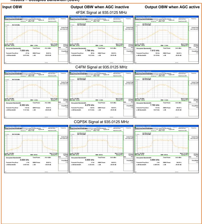
Date Issued: 09 July 2018 Project No.: 16898 Revision No.: 0 **Input OBW Output OBW when AGC inactive Output OBW when AGC active** HDQPSK Signal at 935.0125 MHz Ref Offset 43.8 dB Ref 45.00 dBm Ref Offset 43.8 dB Ref 45.00 dBm Center Fi 935.012500 M Center Fr 935.012500 M Center Fi CF Ste 2.500 kH CF Ste 2.500 ki CF Step 2.500 kH Occupied Bandwidth
