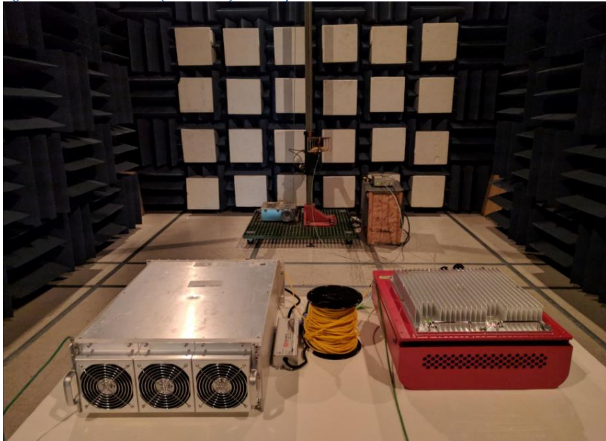
Figure 2: Radiated Emissions (Above 1GHz) Test Setup
