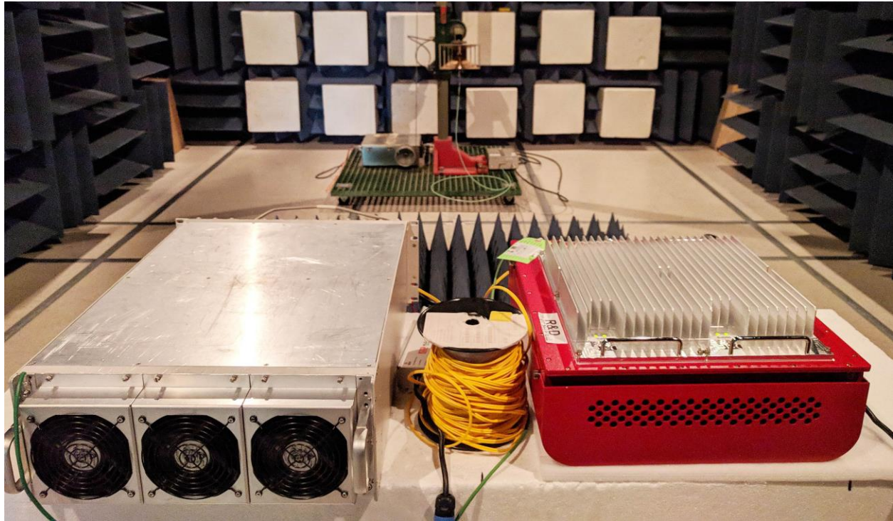
Figure 2: Radiated Emissions (Above 1GHz) Emissions Test Setup
