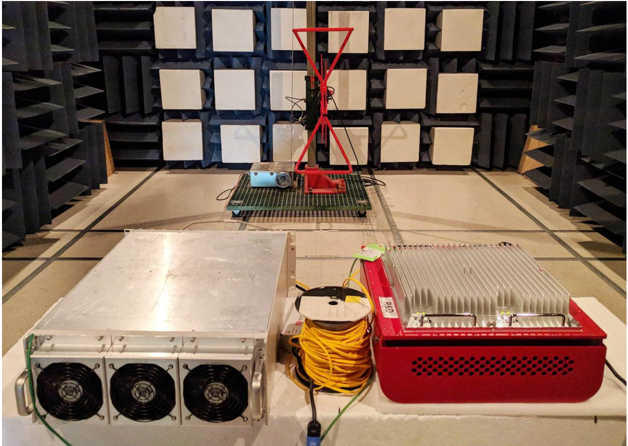
Figure 1: Radiated Emissions (Below 1GHz) Emissions Test Setup
