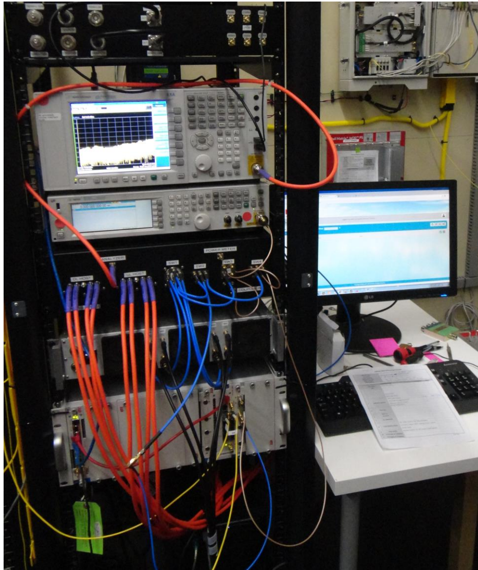
Figure 3: Conducted Test Setup – Rack equipment
