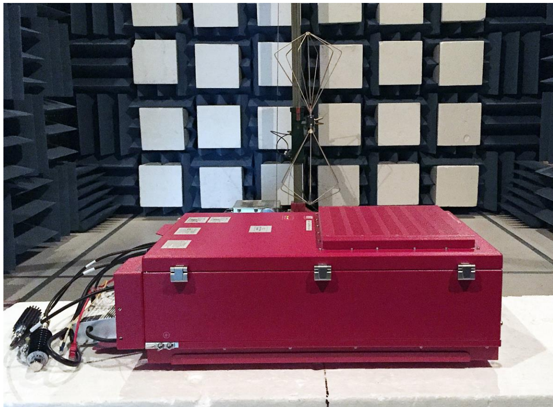
Figure 2: Radiated Emissions (30 to 250MHz) Test Setup
