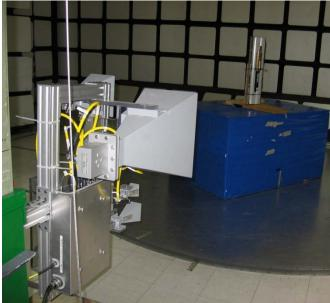
Antenna Conducted Test Setup
