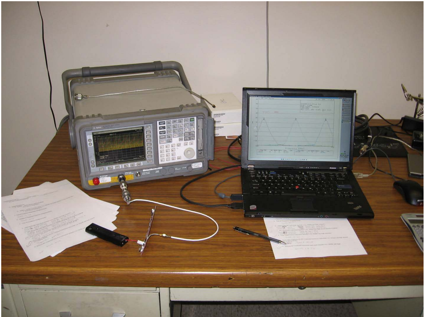
Figure 15 Test Setup for Carrier Frequency Separation
