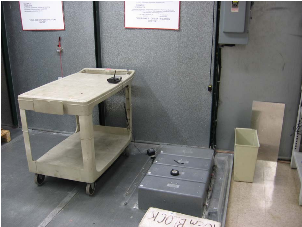
Figure 1 Test Setup for Conducted Emissions
