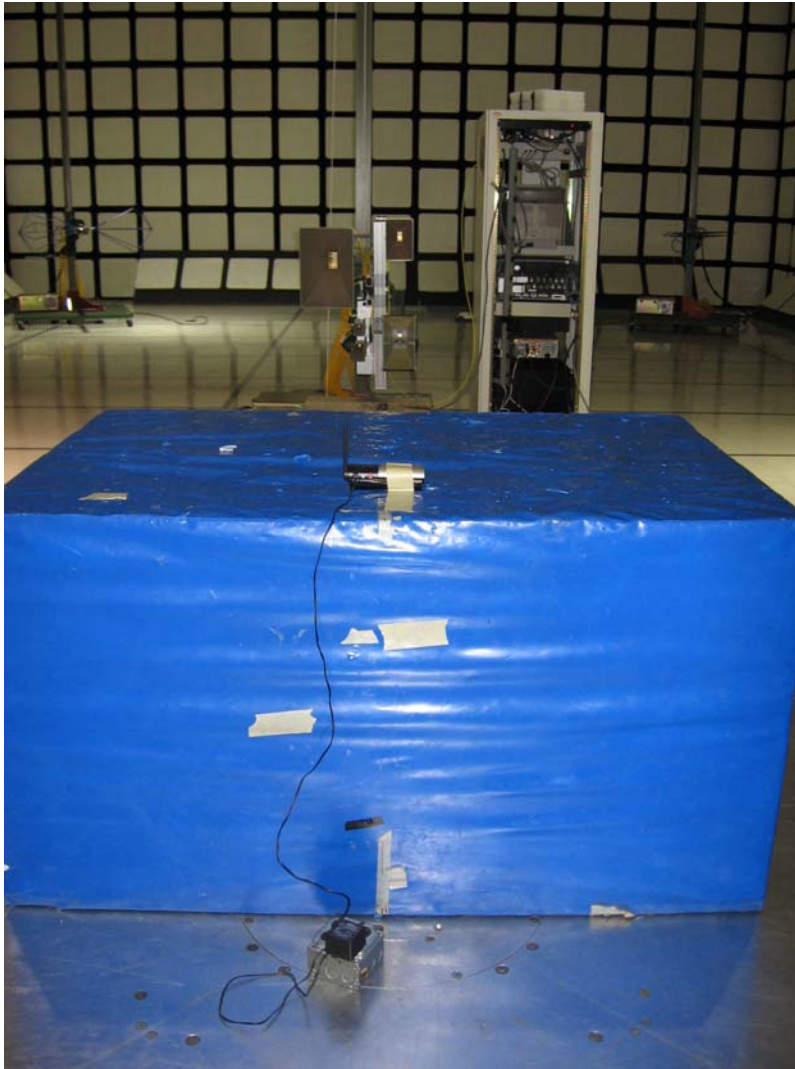
Figure 3 Test setup for Radiated Emissions
