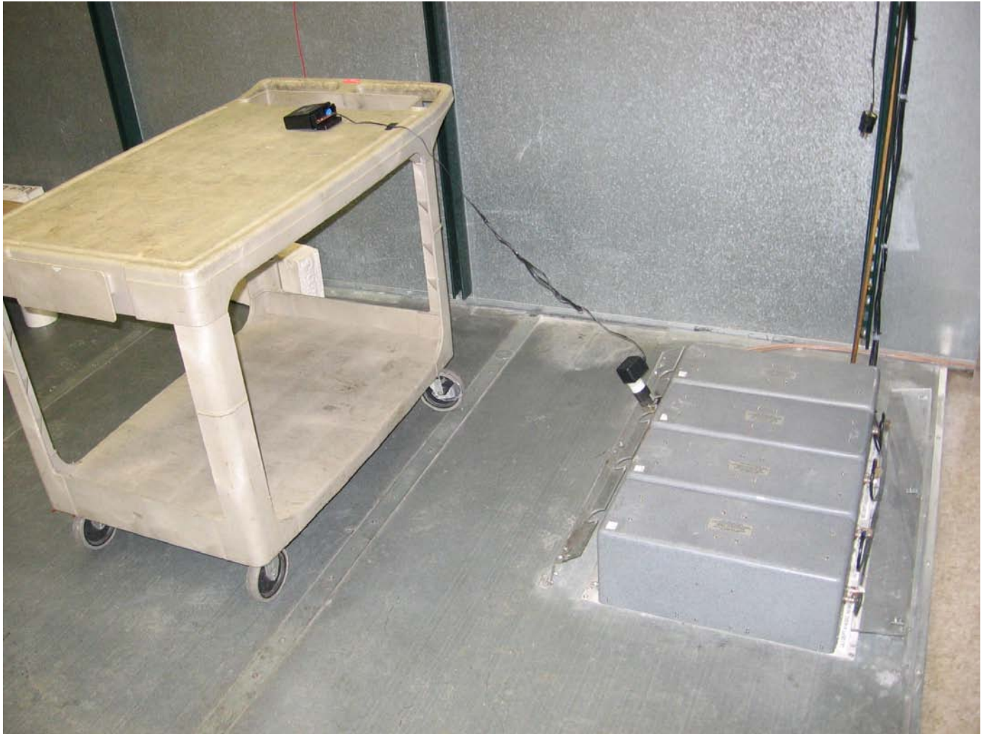
Figure 1 Test Setup for Conducted Emissions
