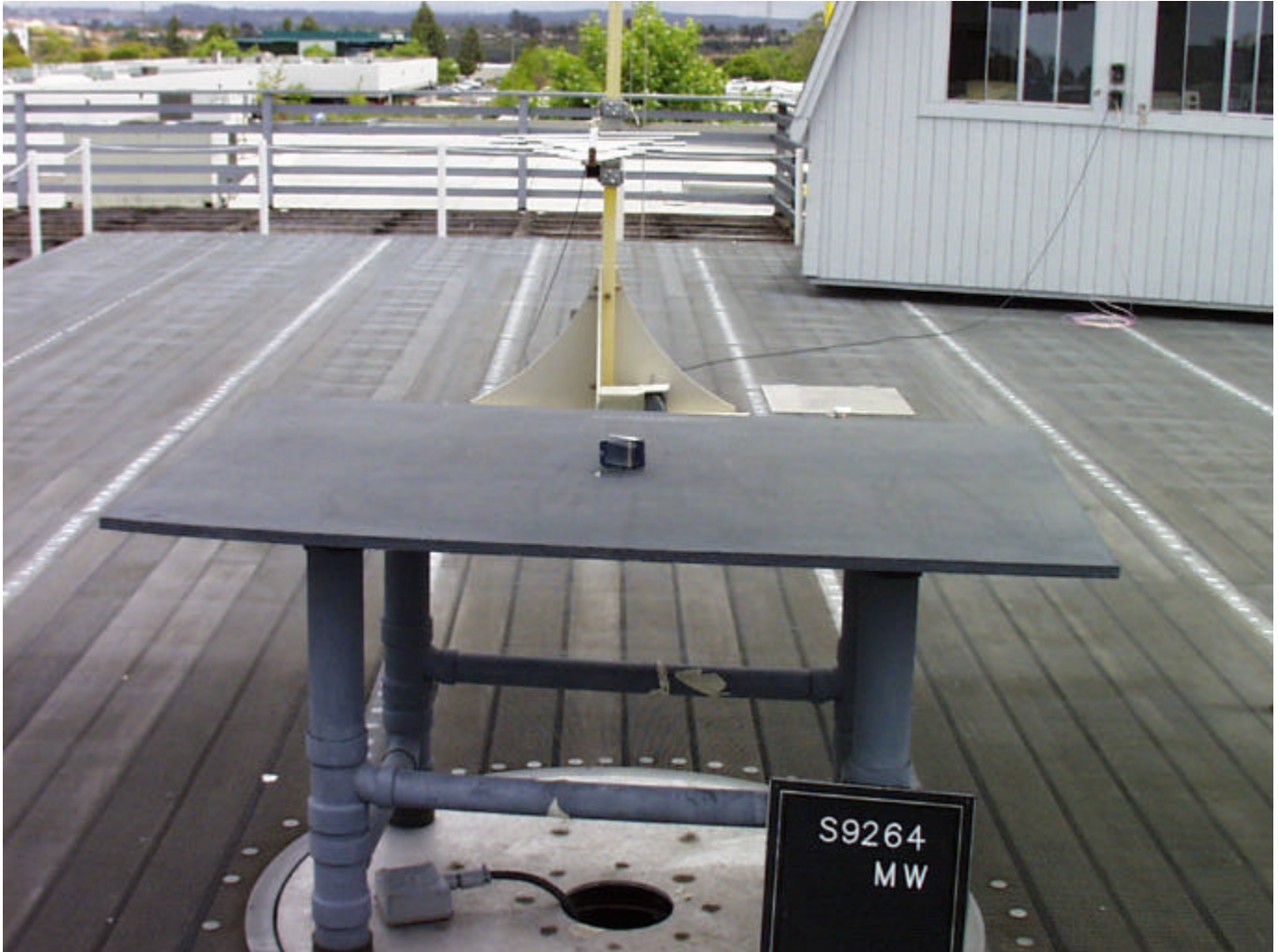
Photograph of Test Setup: Radiated Emissions 30 MHz - 1000 MHz
