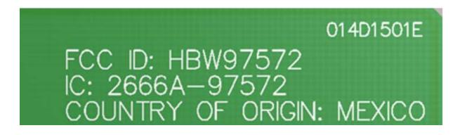
The label will be located in the top righthand corner of the printed circuit board via silkscreen.
