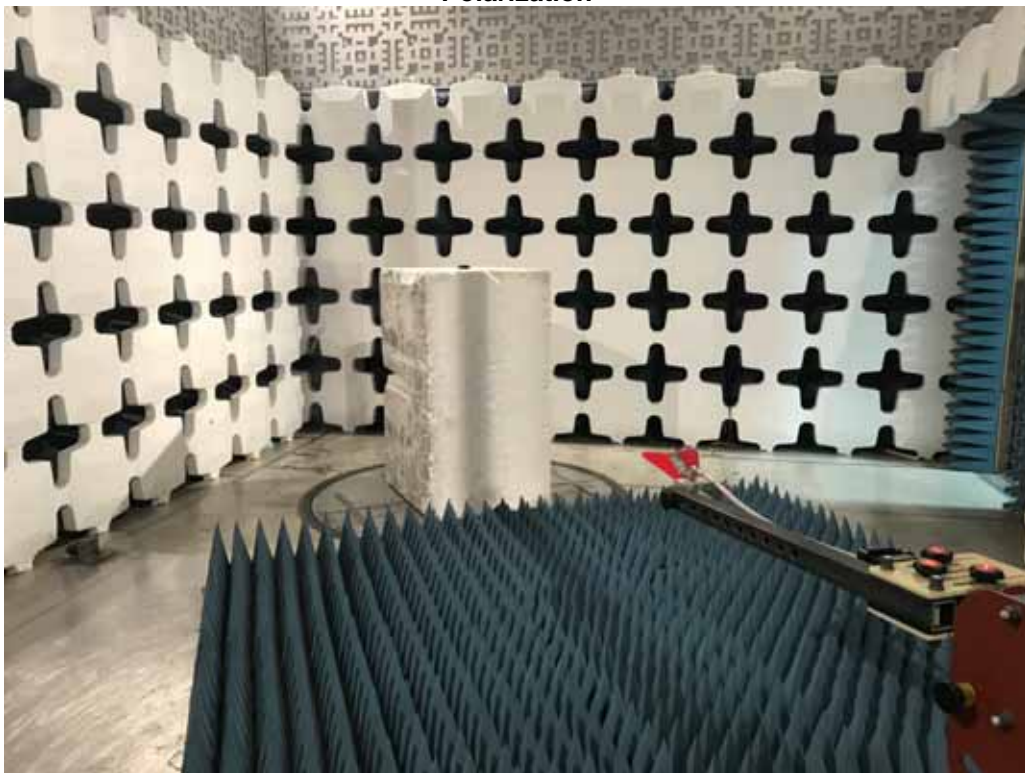
Figure 5 - Test Setup for Radiated Emissions, 1GHz to 4.5GHz – Vertical Polarization
