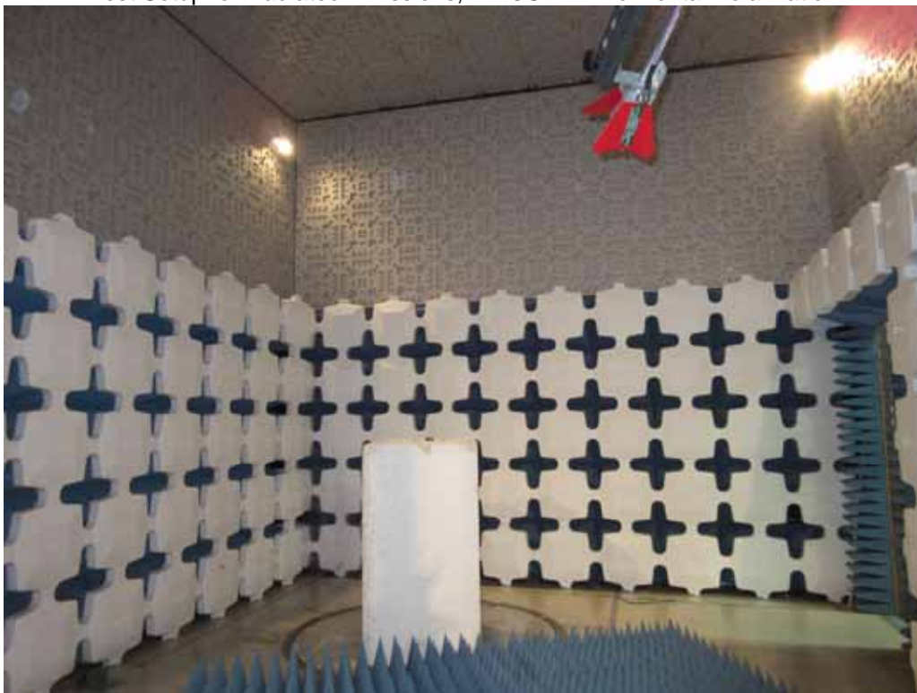
Test Setup for Radiated Emissions, 1-4.5GHz – Vertical Polarization
