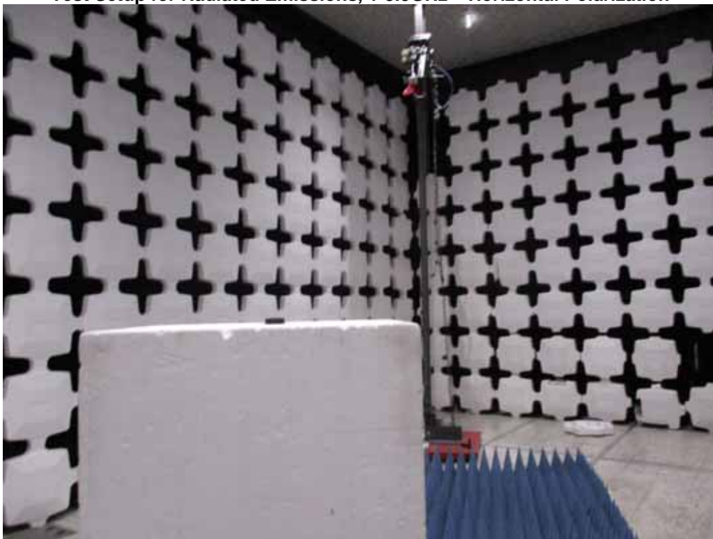
Test Setup for Radiated Emissions, 1-3.5GHz – Vertical Polarization
