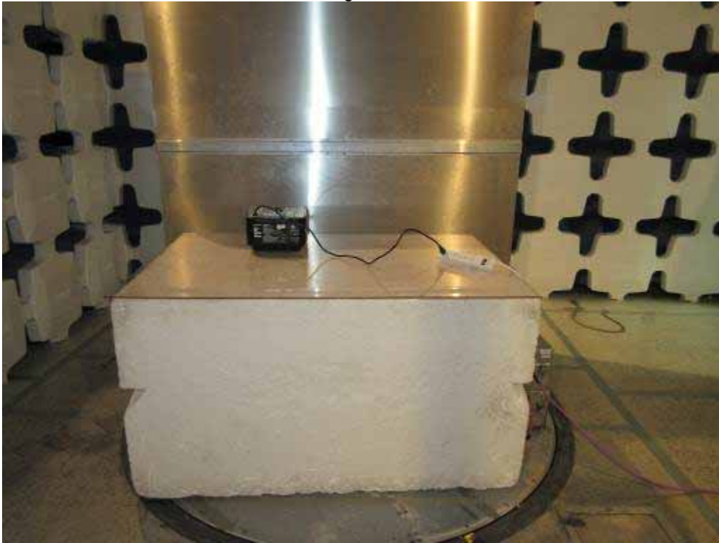
Test Setup for Conducted Emissions
