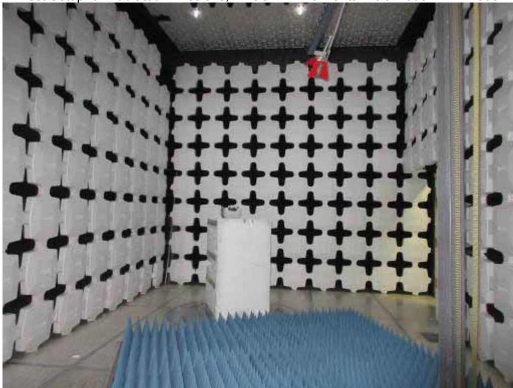
Test Setup for Radiated Emissions, 1-10GHz – Vertical Polarization - Tx Mode
