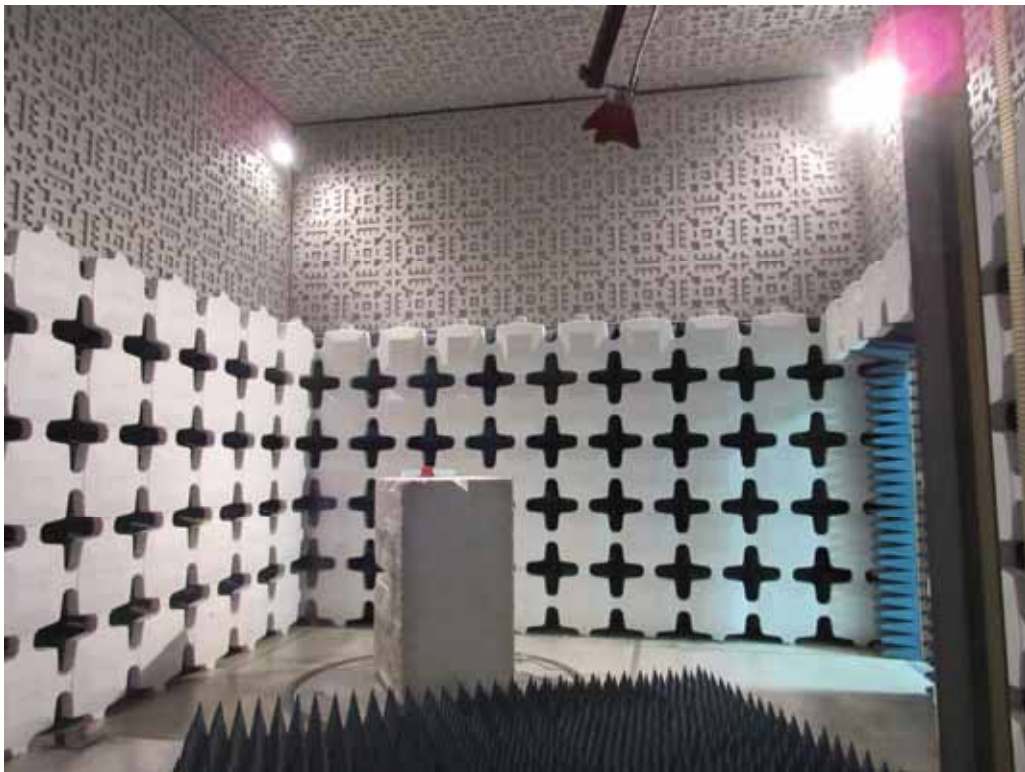
Test Setup for Radiated Emissions, 1 to 18GHz – Vertical Polarization
