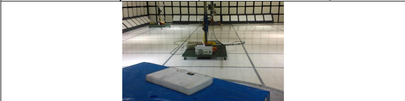
Radiated Emissions setup
