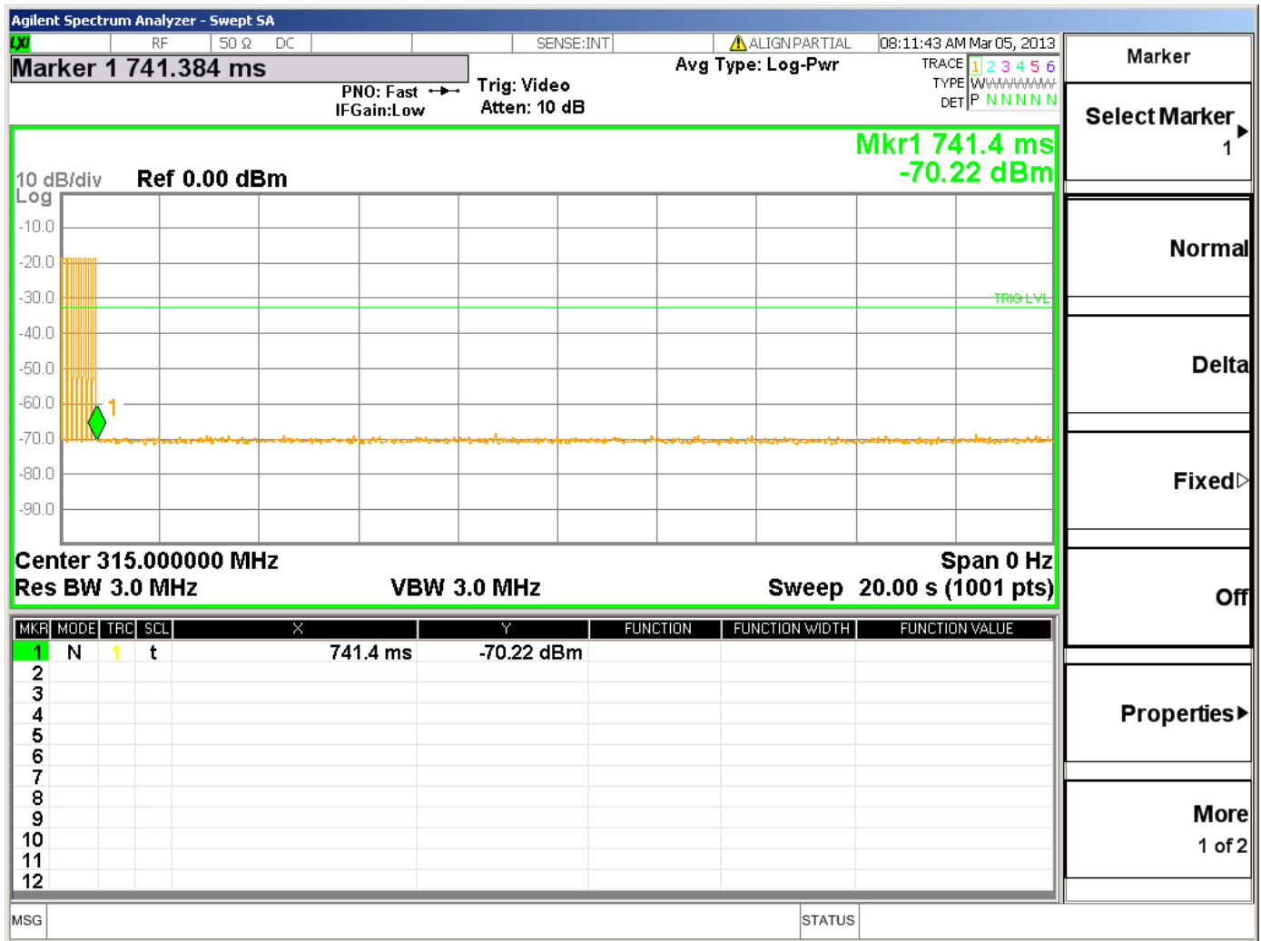
Figure 8 Cease Operation Graph 315MHz
