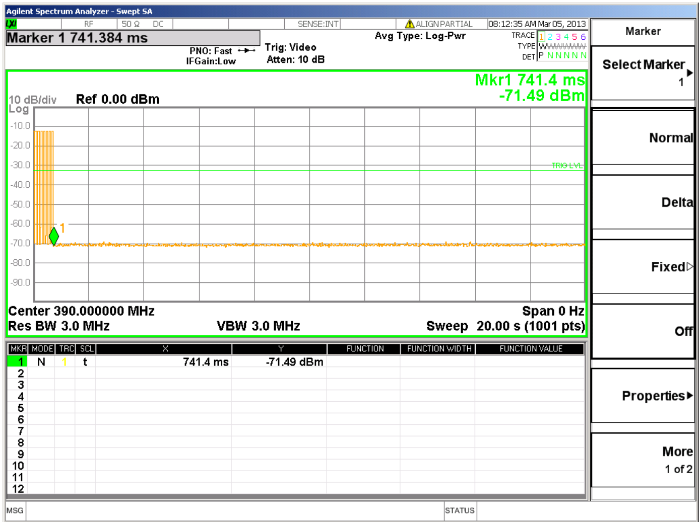
Figure 9 Cease Operation Graph 390MHz
