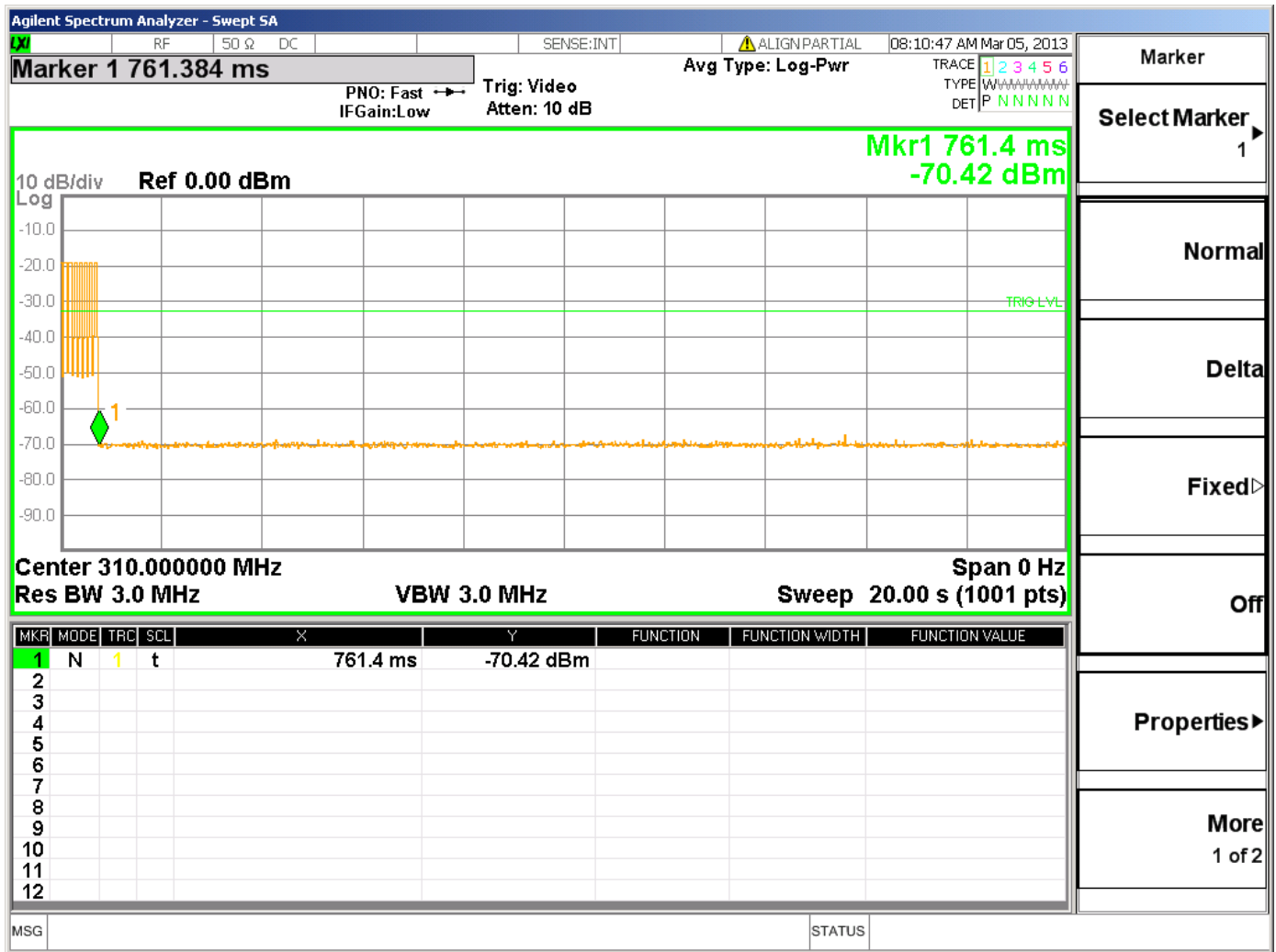
Figure 7 Cease Operation Graph 310MHz
