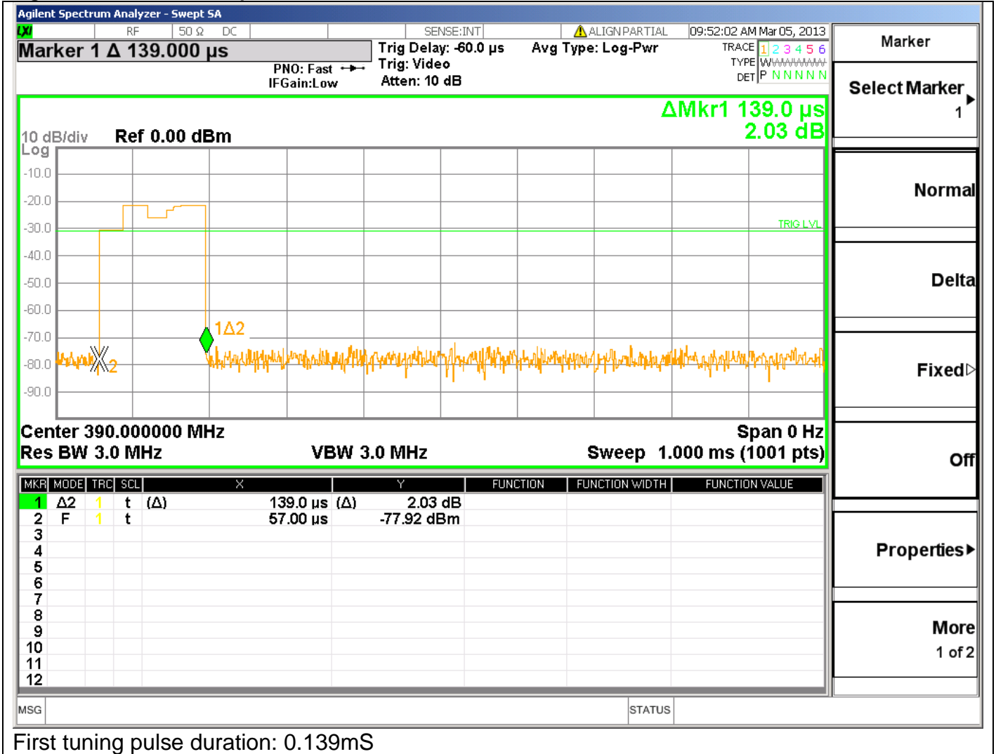
Figure 28 Pulse Train Graphs for 390MHz
