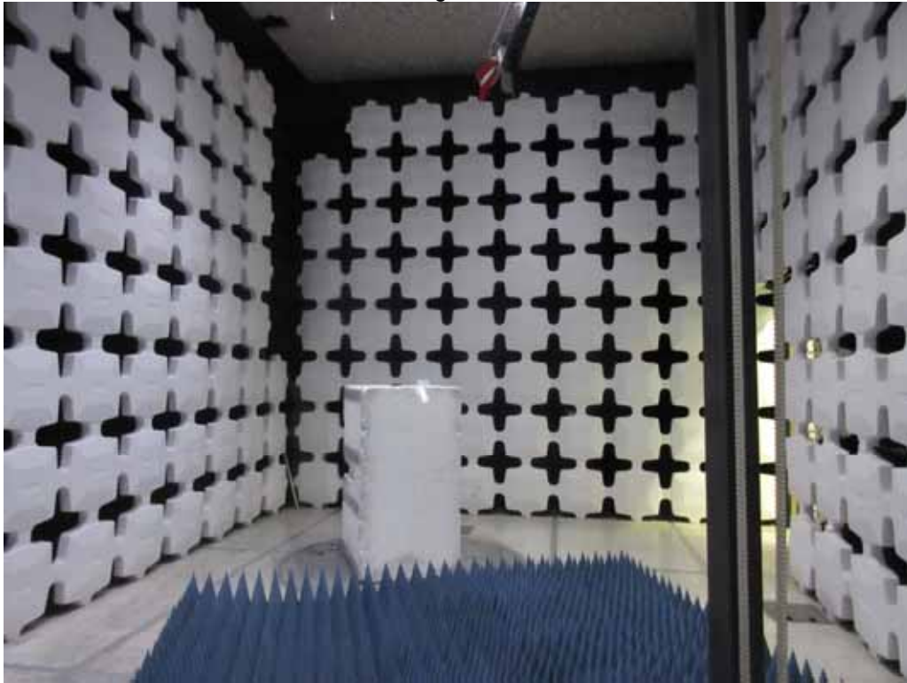
Test Setup for Radiated Emissions, 1 to 4GHz – Horizontal Polarization
