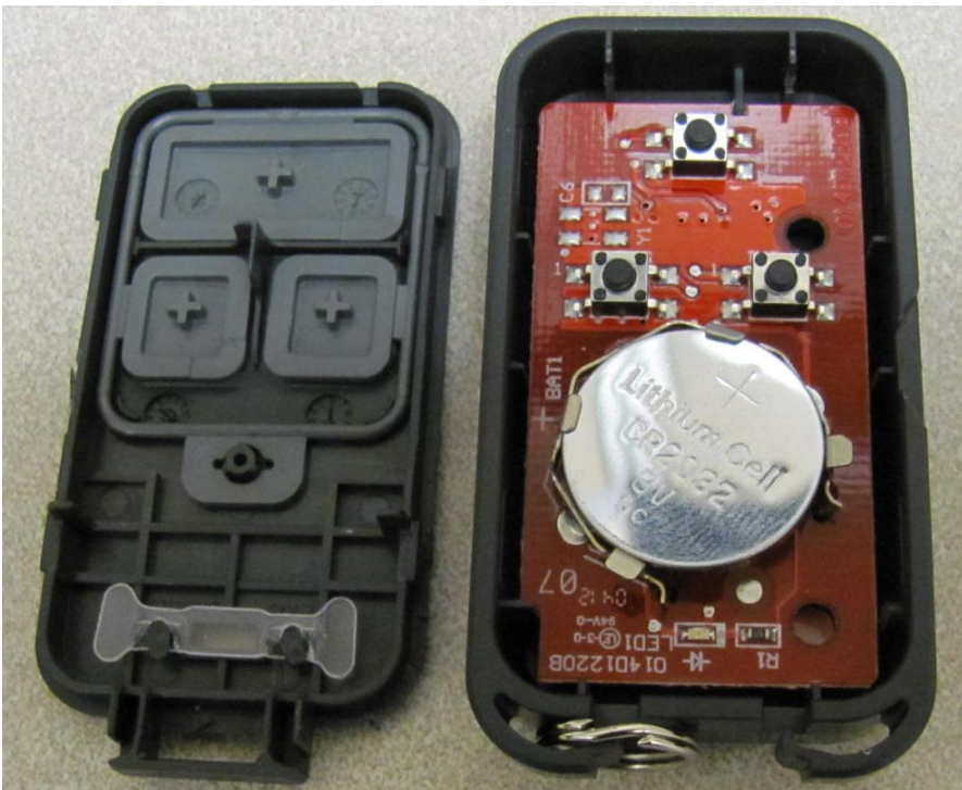
Internal showing the RFID passive coil (the white stick on inside the enclosure)
