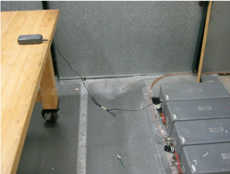
Figure 1 Test Setup for Conducted Emissions
