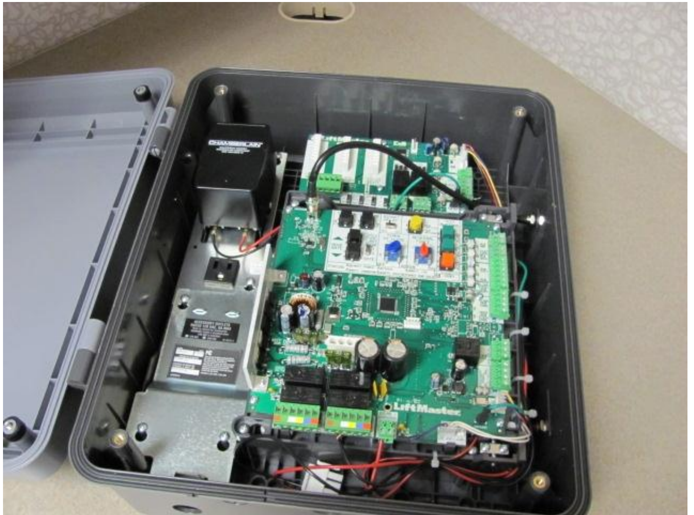
Main PCB Top Inside Enclosure
