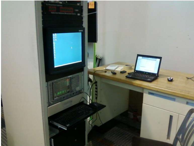
Figure 35 Test Setup for Cease Operation, Pulse Train, and Bandwidth
