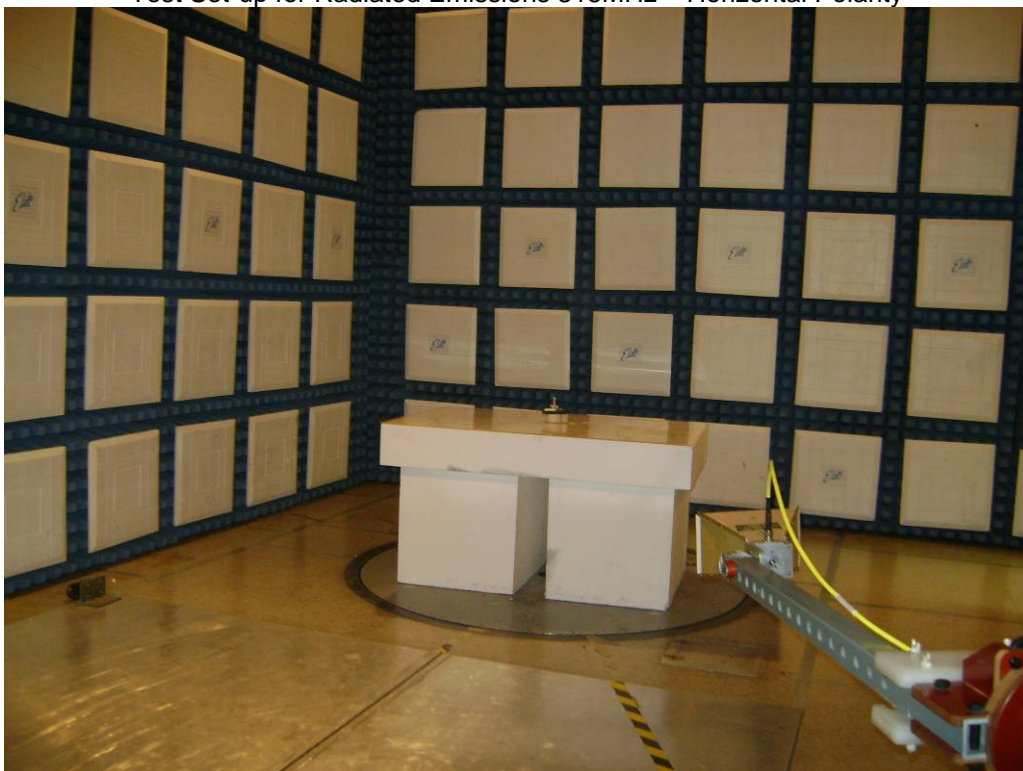
Test Set-up for Radiated Emissions 315MHz – Vertical Polarity
