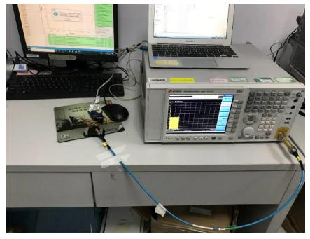
1.2 Conducted Emissions at Mains Terminals (150kHz-30MHz) Test Setup
