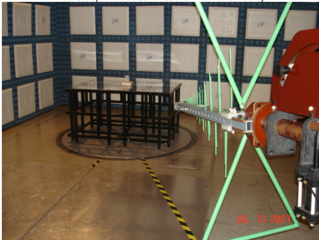
Test Set-up for Radiated Emissions – Vertical Polarity
