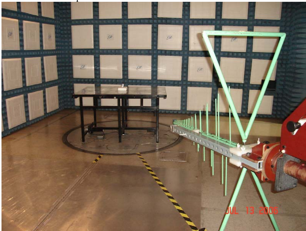
Test Set-up for Radiated Emissions – Horizontal Polarization
