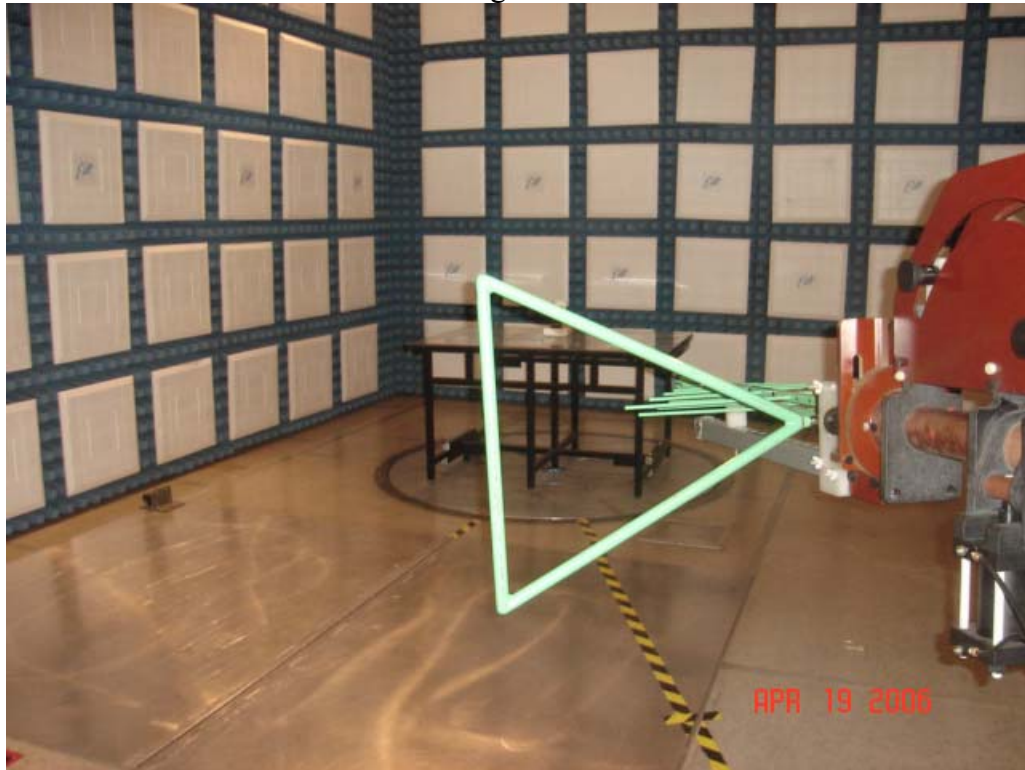
Test Set-up for Radiated Emissions – Horizontal Polarization
