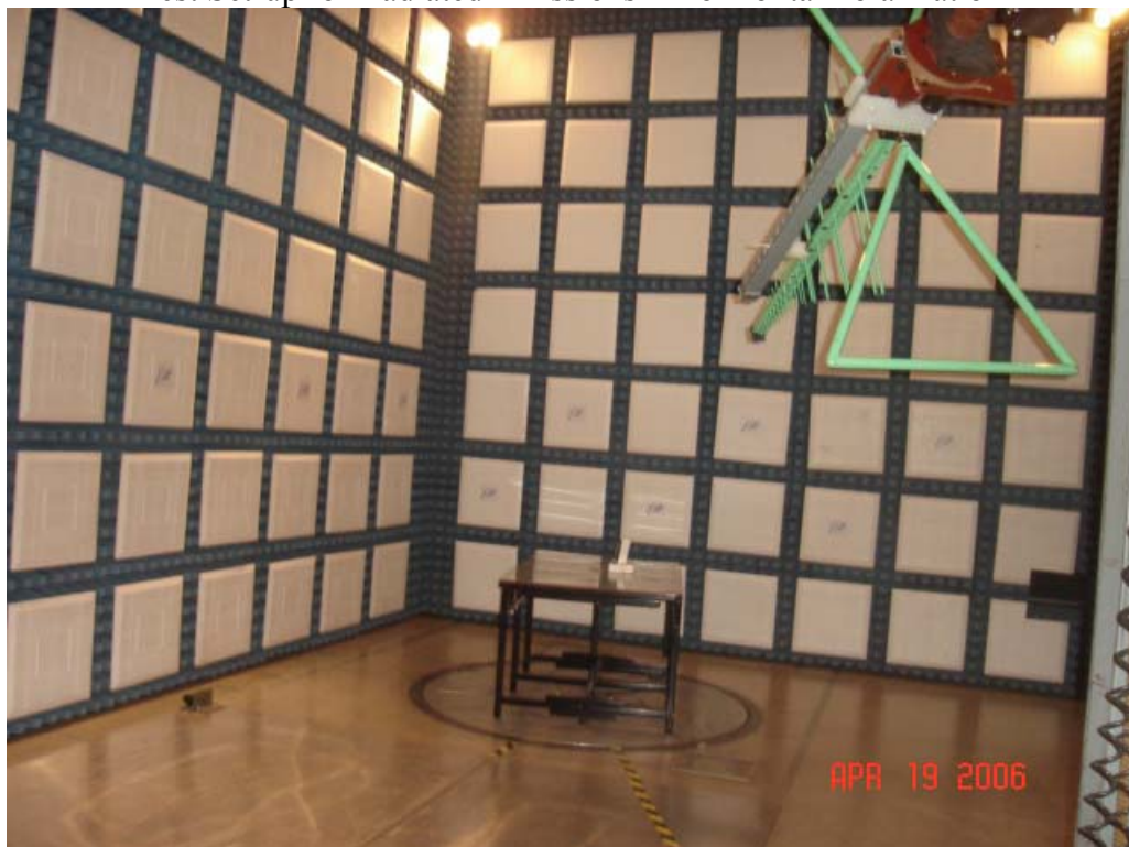
Test Set-up for Radiated Emissions – Vertical Polarization
