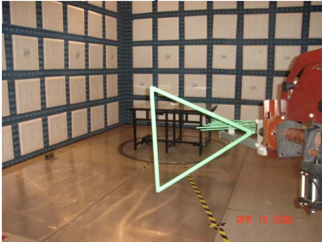
Test Set-up for Radiated Emissions – Horizontal Polarization
