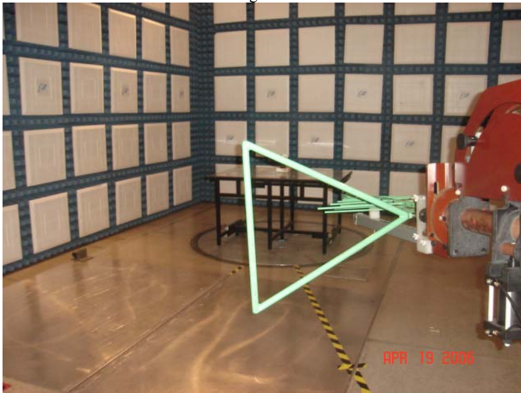
Test Set-up for Radiated Emissions – Horizontal Polarization
