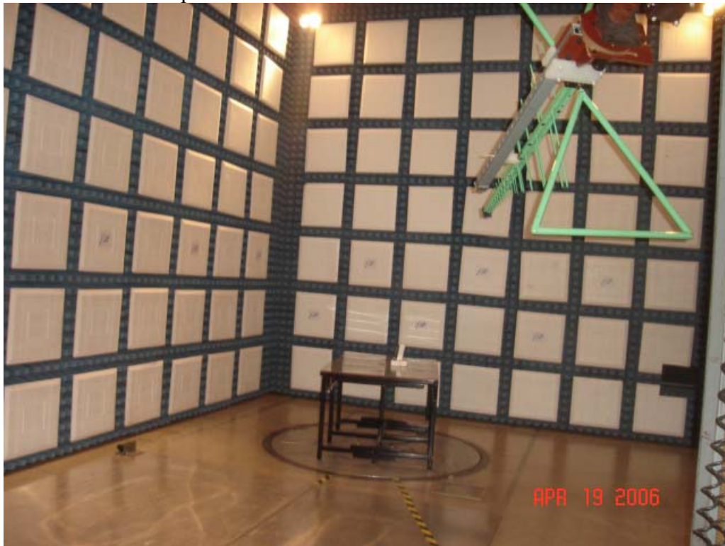
Test Set-up for Radiated Emissions – Vertical Polarization
