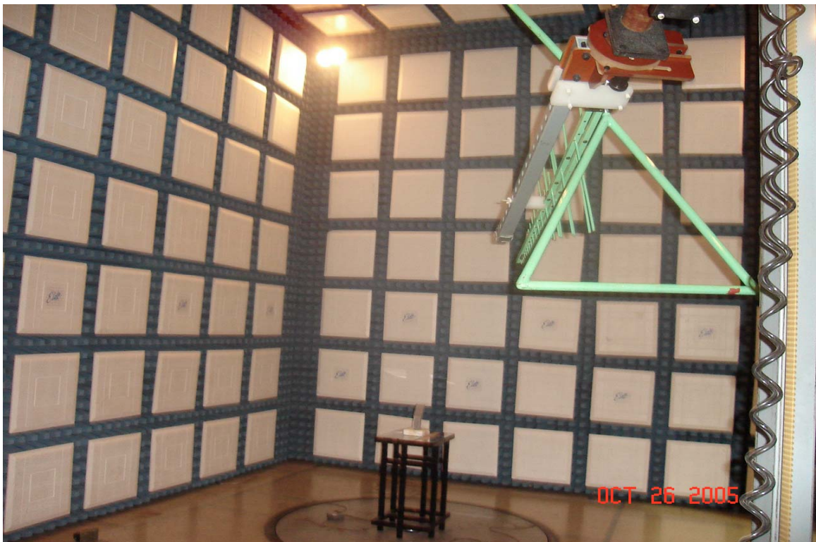
Test Set-up for Radiated Emissions Vertical Polarity
