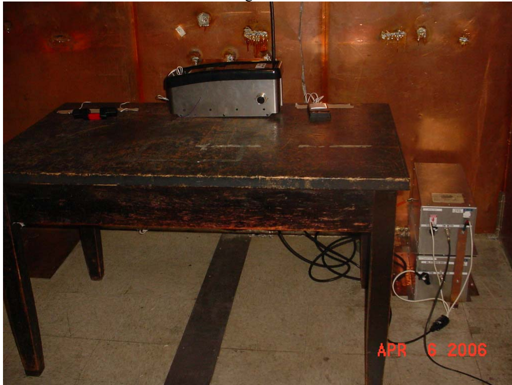
Test Set-up for Conducted Emissions
