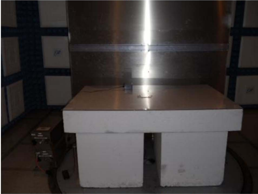
Test Setup for Conducted Emissions, 150kHz to 30MHz
