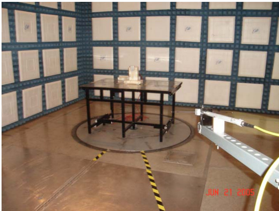
Test Set-up for Radiated Emissions Horizontal Polarity
