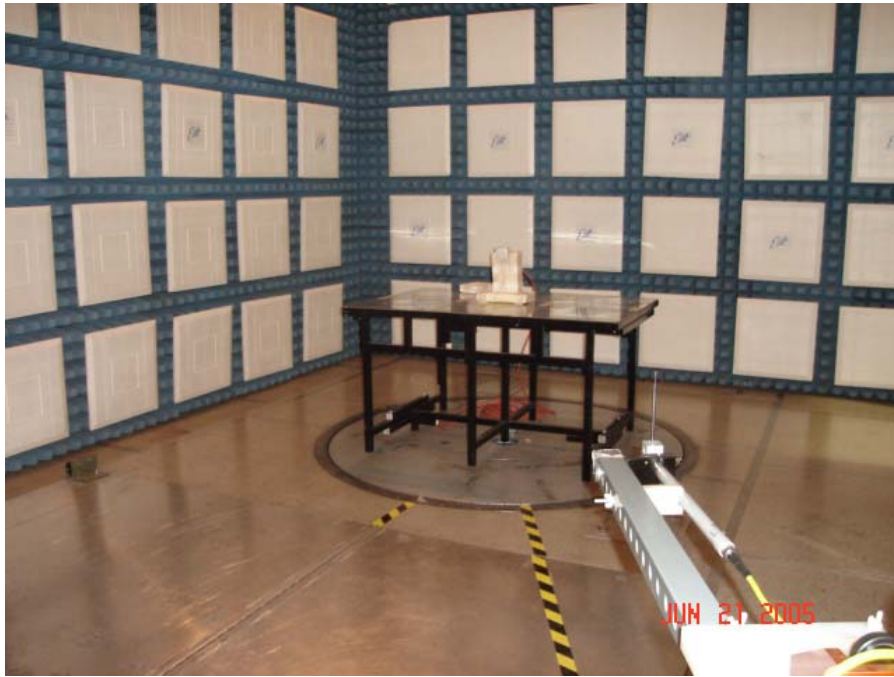
Test Set-up for Radiated Emissions Vertical Polarity
