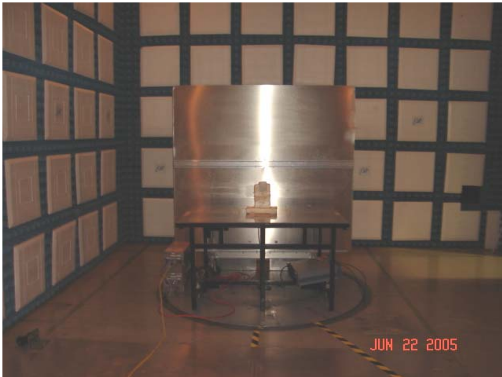
Test Set-up for Conducted Emissions
