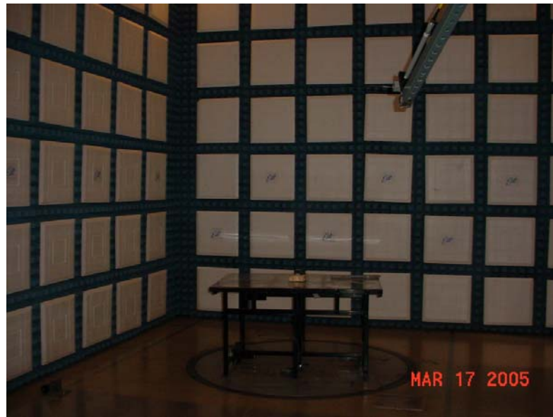
Test Set-up for Radiated Emissions Horizontal Polarity
