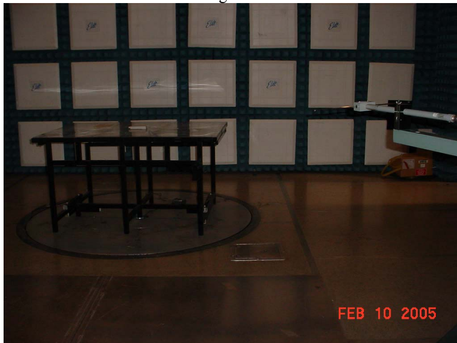
Test Setup for Highest Radiated Emissions Measurement Horizontal Polarity
