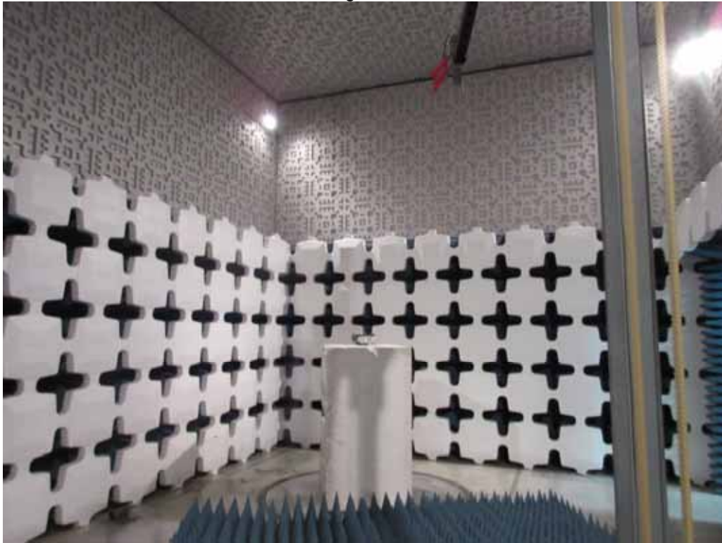
Test Setup for Radiated Emissions, 1 to 5GHz – Horizontal Polarization
