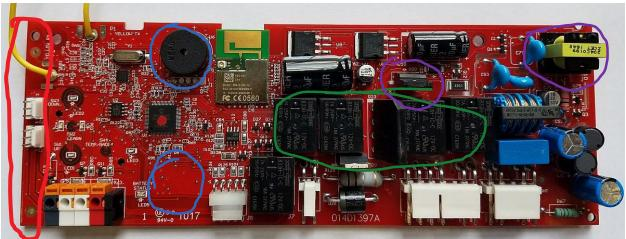
Circled in red is the area of the board added with the new PCB connectors.
