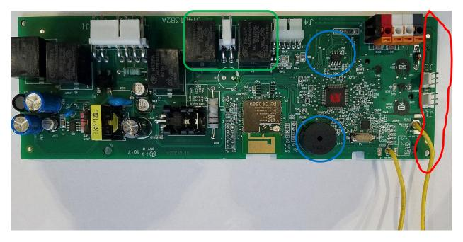
Circled in red is the area of the board added with the new PCB connectors.
