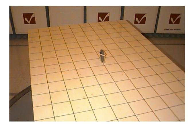
View of the Remote Control transmitter during the Radiated Emissions tests. This view shows the orientation of the product where the maximum signal levels were present (vertical polarity). In order to cause the remote transmitter to run continuously, a small plexiglass fixture can be seen which pushes a plunger down on the appropriate button to activate transmission.
