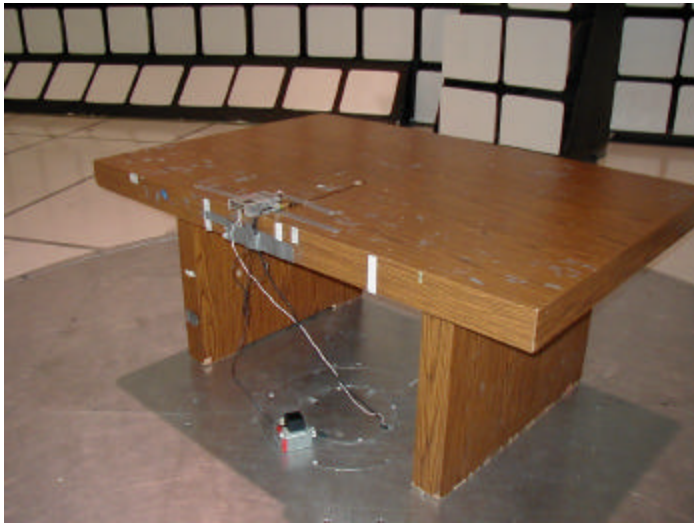
Radiated Emissions 10M Chamber
